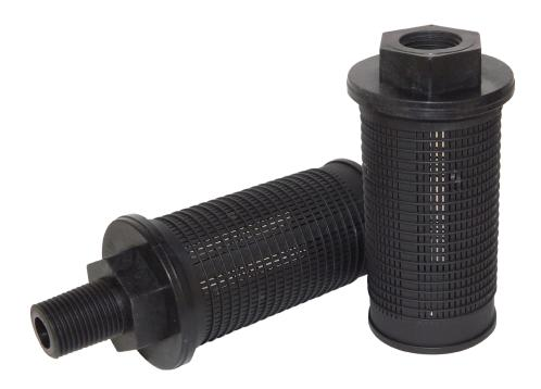
These all nylon, suction strainers are ideal for use where stainless steel or other metal strainers may corrode or maybe a non-metal strainer that is low flow and low cost can be used. Such applications include, water, including seawater and de-ionized water, medical/pharmaceutical, general industrial, chemical, and coolant/lubricant and are rated to 290 degrees F. They are installed in the suction line, in-tank, whose purpose is to protect the pump for flow rates up to 3 gpm.
